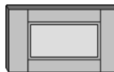
2 1/4" Stile with 1 1/2" Rail (codes starting with "D")
