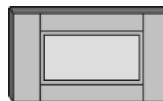
2 1/4" Stile with 1 1/2" Rail (codes starting with "D")
