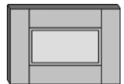
2 1/4" Stile and Rail (all codes with suffix "HG")
