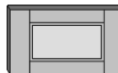
2 1/4" Stile with 1 1/2" Rail (codes starting with "D")
