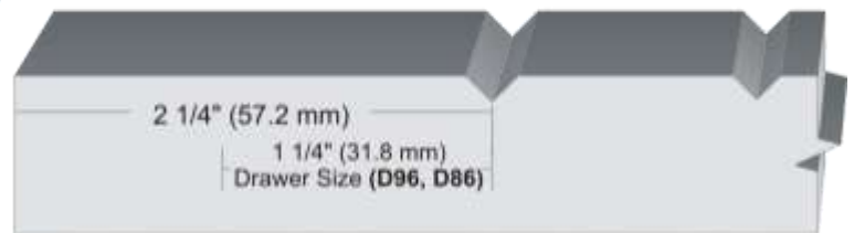
M96 V-Groove Panel & V-Groove Through Stile and Rail M86 V-Groove Raised Panel (Square Pattern Routed Only)
